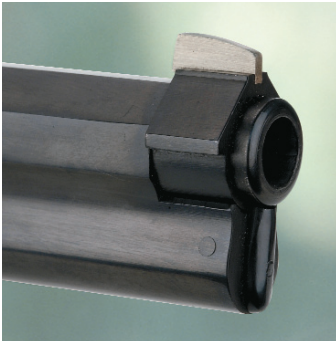
Sights consist of a white metal blade front and folding leaf rear mounted on the barrel with ladder-type elevation marked "2" through "8" in increments of one.
